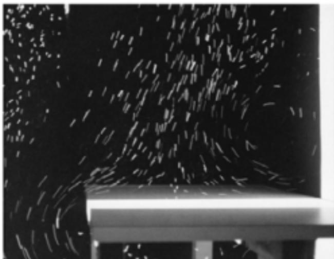
**Figure 4: Helium bubble testing of airflow patterns**
