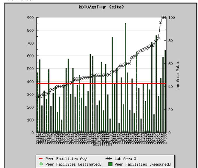
**Figure 1: Lab site energy intensity for climate zone 5A (from Labs21 benchmarking tool)**
